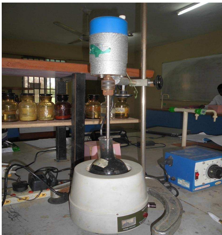
Fig. 2. Experimental set-up for the extraction of manganese and zinc from the waste Zn-carbon batteries
